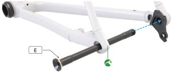
Apply grease to the rear thru-axle (E) threads, then install the wheel, thru-axle, and conical washer. Using a torque wrench and 6 mm hex bit, torque the thru-axle to 15 Nm / 133 in-lbf.
