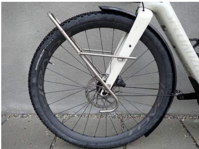
front racks can be combined with fenders - mounting the struts at the fork dropout may require special attention/solutions
