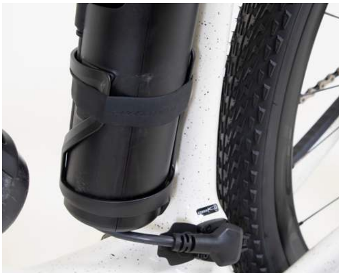
when connecting a Range Extender battery, always use the supplied Zee Cage and always secure it with the retention band.
