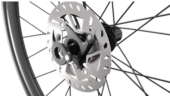
Speed Sensor magnet, centerlock design
