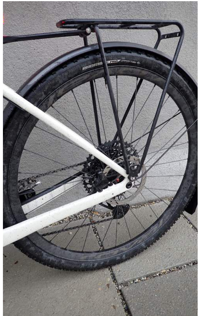
the tubus Vega Classic offers ample of clearance for the DryTech 52c fenders
