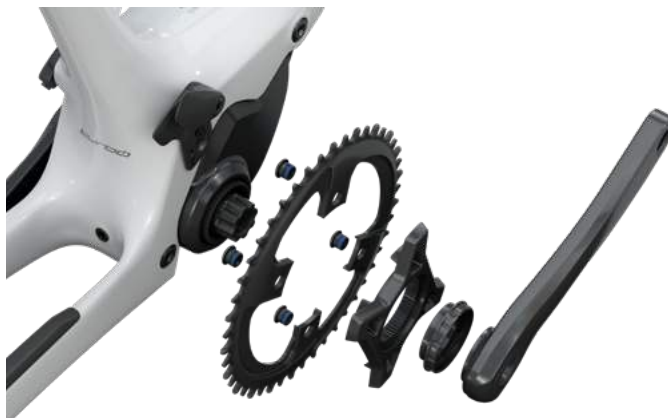
the spider accepts 107 BCD chainrings; matching SRAM X-sync chainrings are recommended
