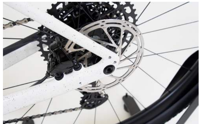
flat mount 2-piston calipers, paired with 160 mm rotors
