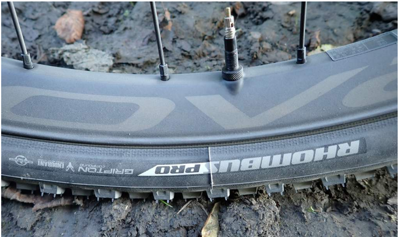
Rhombus Pro 47c tire on Roval Control Carbon rim, tubeless
