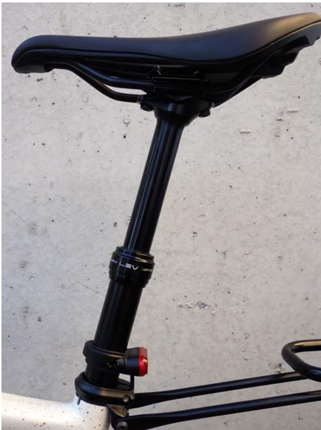
a Kind Shock LEV Integra 27.2 dropper post with 100 mm of travel, installed in a size 56 frame
