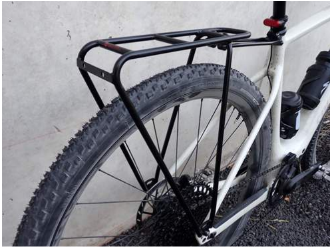
the 29" version of the Vega Classic is 2 cm higher than the 28" version, providing more clearance for wide tires, fenders and long panniers.
