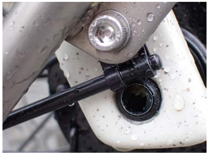
here, the drive side fender strut clamp is combined with the lower rack mount screw
