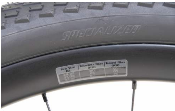
Terra rims give pressure recommendations
