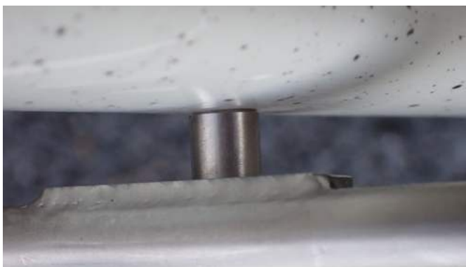
to adapt to the fork width, the supplied 8 mm washers are used at both top mount points
