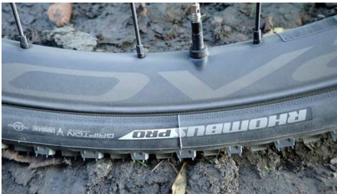
Rhombus Pro 47c tire on Roval Control Carbon rim, tubeless
