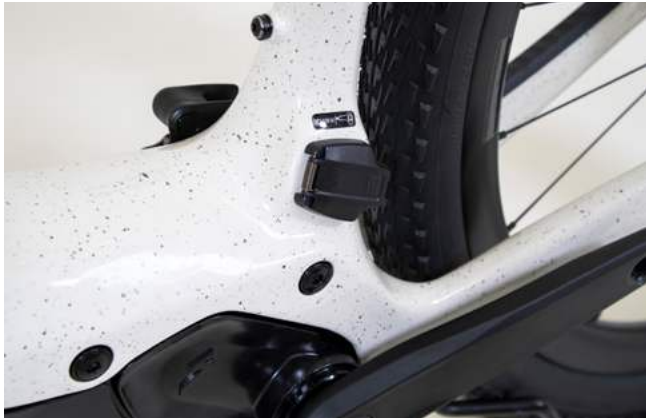
Charge port closed (riding & washing)
