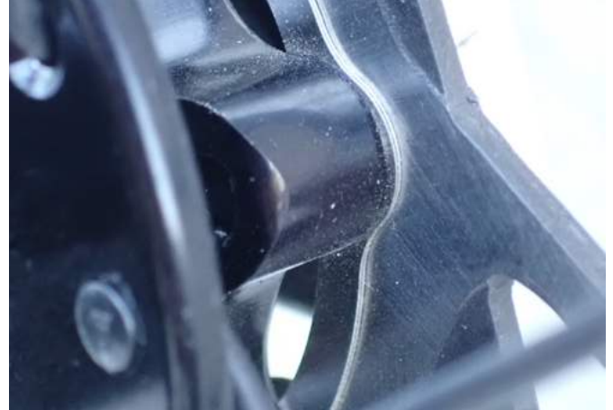
a six-bolt rotor on a second wheelset, using 2x 0.2 mm disc shims for alignment
