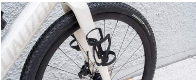
Specialized Zee cages, one at each fork blade
