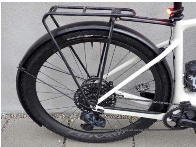
rear rack and fenders share the lower mounting points
