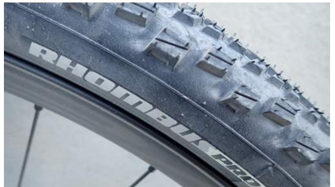
Rhombus Pro 47c tire on Roval Control Carbon rim, tubeless
