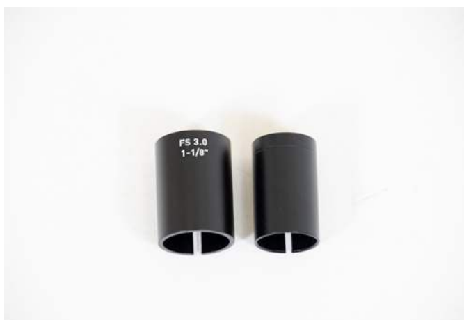
left - optional Future Shock stem shim to mount a std. 1 1/8 stem note: FS 3.0 cartridges do not require a shim when mounting a Future Stem
