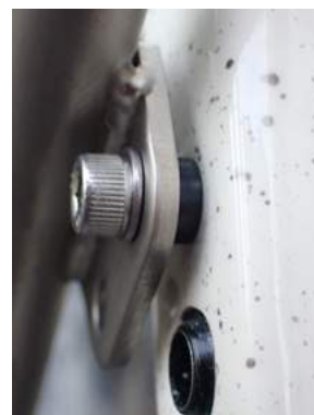
to adapt to the fork width, 3 mm washers (not supplied) are used at both lower mount points
