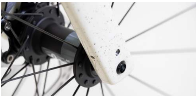
thread to fix fender strut (drive-side)
