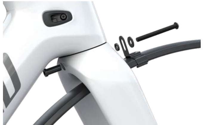
the fork crown features a central mounting hole to install the fender - hardware is not included
