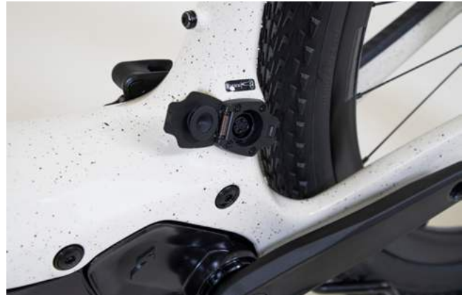
Charge port open (charging, connecting RE, drying/cleaning)
