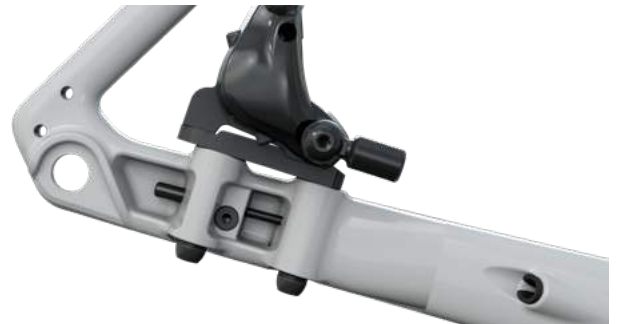
Speed Sensor in non drive-side chainstay
