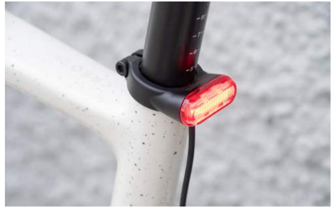
the Lupine C14 is bright and nicely integrated into the seatpost collar
