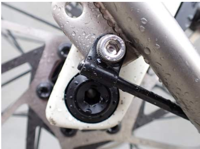
on the non-drive-side, fender strut and rack use a shared mounting point, which means the strut clamp needs to be removed before inserting/removing the thru axle; further, the fender strut touches the rack rail
