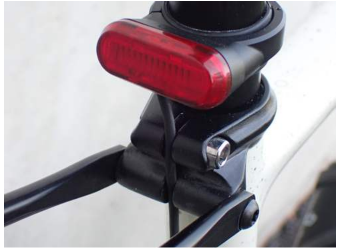
the two forward-facing struts ensure good stiffness when loading the rear rack to the maximum.
