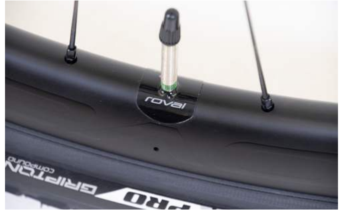
install the supplied sticker to prevent the valve stem from rattling / vibrating
