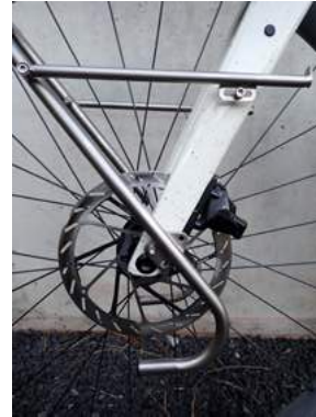
the pannier rail should be horizontal as shown in this image, but a slight angle (left image) is not a problem.
