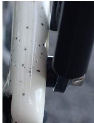
at the dropouts, two 3 mm spacers were used so that the rack legs clear the seatstays
