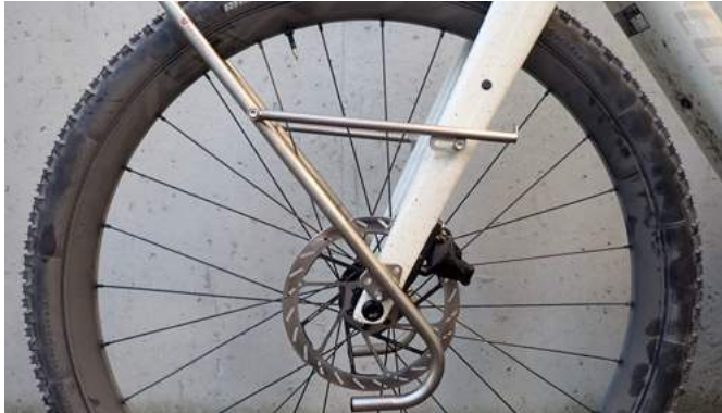
the tubus tara is a functional and clean solution; here, the pannier rail is not perfectly horizontal for clearance reasons of the thru axle (see below).
