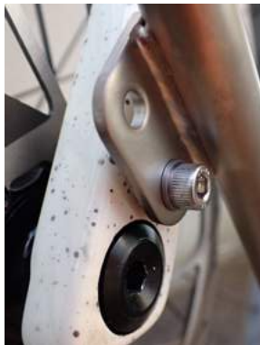
note that in this mounting position the pannier rail is not perfectly horizontal (see above), but the thru axle can be inserted/removed without unscrewing the lower mount and loosening other bolts.
