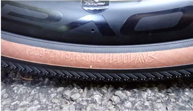
Sawtooth 42c tire on Roval Terra C rim, with tubes
