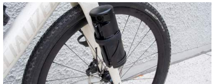
SL Range Extender Battery in Zee cage
