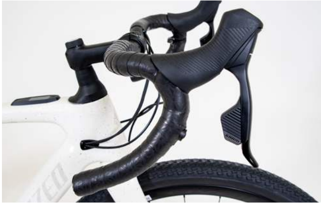
brake lever reach can be adjusted with a 2.5 mm allen key
