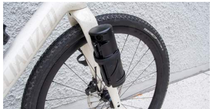
when carrying a Range Extender battery like this, always use the supplied Zee Cage and always secure it with the retention band.
