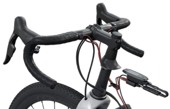
Remote routing to junction box under display
