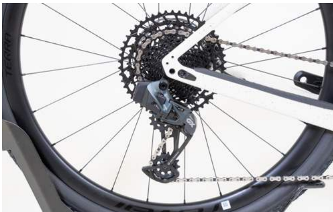
10-50 or 11-50 cassettes for wide gearing range
