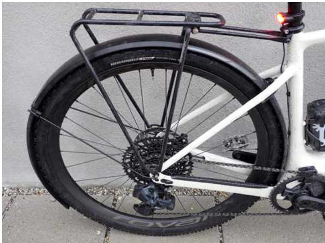
the tubus Vega Classic offers ample of clearance for the DryTech 52c fenders
