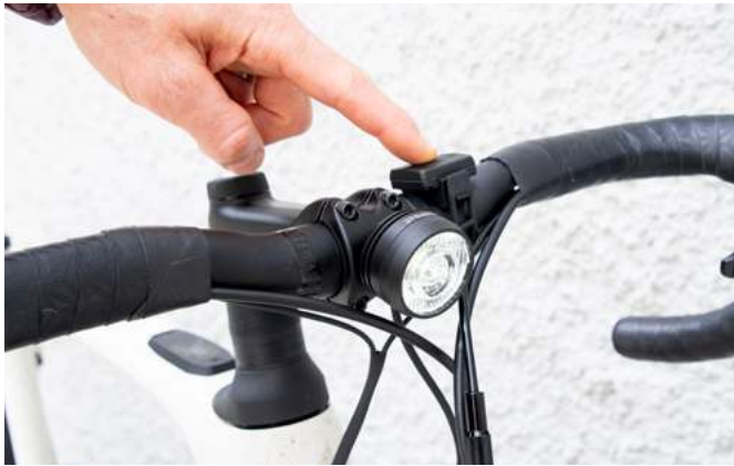
the Lupine SL Nano F is available as Bluetooth version to control the lamp with a remote
