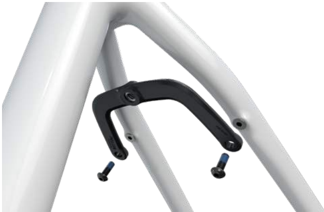
the rear triangle uses the supplied bracket to install the fender
