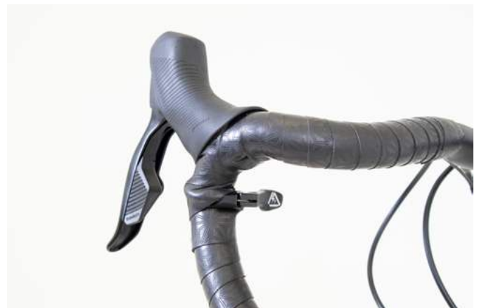
dropper post lever comes pre-installed in intended position
