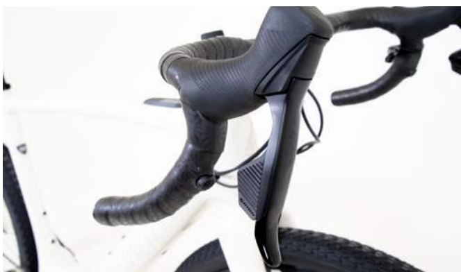
Possible remote location under hoods - leave a sufficient gap for hands (3-4 cm)
