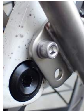
note that in this mounting position the pannier rail is perfectly horizontal (see above), but the thru axle cannot be inserted/removed without unscrewing the lower mount and loosening other bolts.
