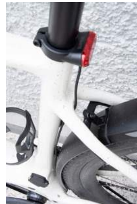
the rear light cable is routed along the back of the seat tube, using supplied cable clips with self-adhesive patches
