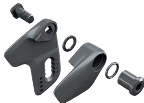
the chainguide has markers to height-adjust it for 42-48t chainrings
