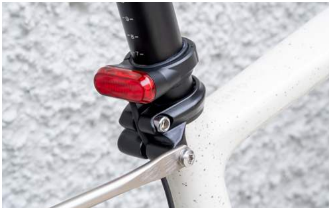
the Lupine C14 SP is a good solution if a seatpost clamp with integrated rack mounts is installed
