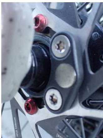
6-bolt speed sensor magnet on second wheelset
