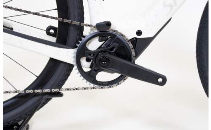
chain guide is adjustable to 42t-48t chainrings
