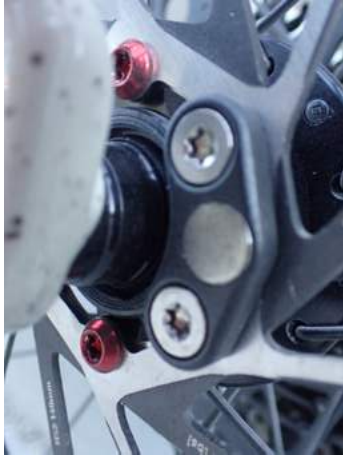
6-bolt magnets work with the system
