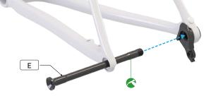
Apply grease to the rear thru-axle (E) threads, then install the wheel, thru-axle, and conical washer. Using a torque wrench and 6 mm hex bit, torque the thru-axle to 15 Nm / 133 in-lbf.
