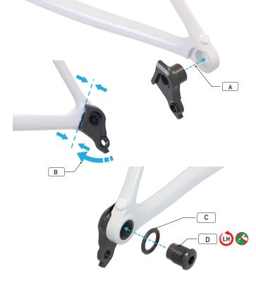
Install the UDH hanger (A) into the frame dropout and rotate it forward until it's completely seated (B) in the hanger pocket or contacts the rotational stop tab.
